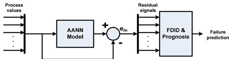
Figure 4: Virtual sensor scheme with FDID and prognosis algorithm as presented in (Hines et al., 1998)
