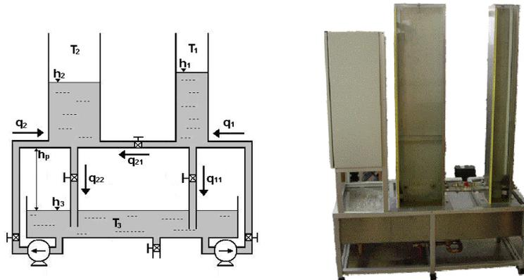
Figure 6: Process flowsheet (left) and image of the laboratory model (right).
