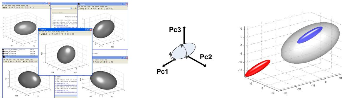
Figure 1: Different PCA models for different process operating regimes(left), and batch prediction (right); rejected batch (red) and accepted batch (blue).
