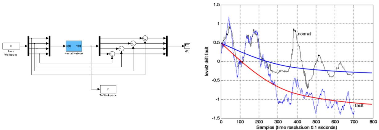
Figure 11: Data reconciliation scheme (left) and detection of slow drift with trend prediction (right)
