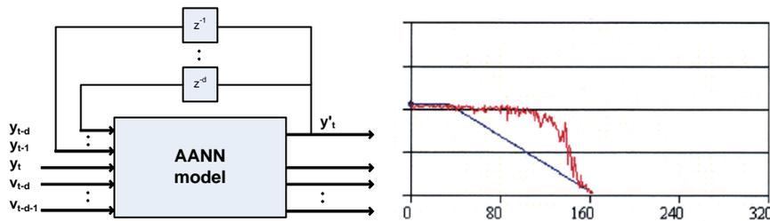
Figure 5: Reconstructed outputs are fed back to the input layer (left) and sensor degradation (right).
