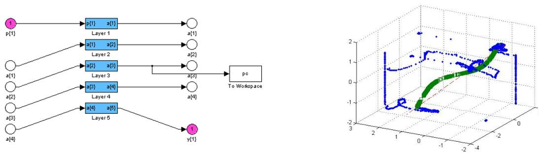
Figure 10: Auto-associative neural network structure in Matlab/Simulink (left) and extracted first NLPC.
