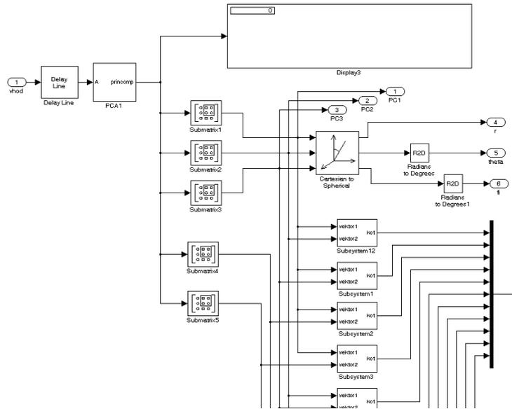
Figure 7: Matlab/Simulink sub-system for PCs batch
