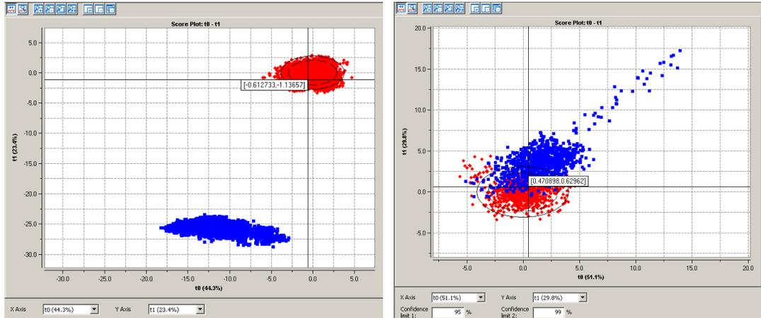
Figure 13: PCA score graph; normal operation (red) and faulty sensor (blue) scores (left), and obvious sensor drift detection at small sensor displacement (right).
